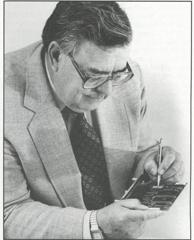
Ron Earp sets the switches on the control card from the system's DSP-2 Digital Signal Processor.
